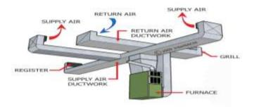
If you have a forced air (aka, "Central Air") heating and cooling system in your home, it can make a world of difference to **make sure that the air is going to the places you want it,** and not to the spaces in the home you don't use. Make sure the thermostat is located in a room that gets good airflow, but seal up vent openings to rooms you don't need.
